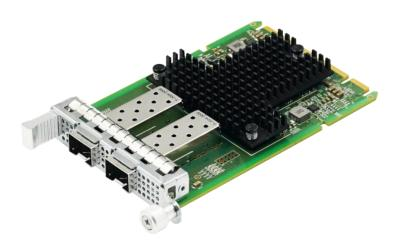
LRES3032PF-OCP is a dual-port optical fiber network adapter with OCP 3.0 SFF structure developed by Shenzhen Lianrui Electronics Co., Ltd. based on the RNP N10 solution of the MUCSE controllers. It adopts the industry-leading intelligent network security control chip, has complete independent intellectual property rights, and realizes a high degree of integration of network and security in product performance.
